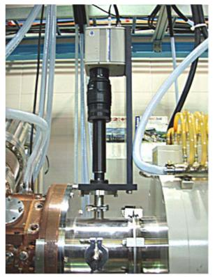
Figure 1: The installation of the CCD beam profile monitor at the PEFP LEBT.
