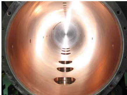
Figure 2: Copper Plated surface : before/after mechanical polishing
