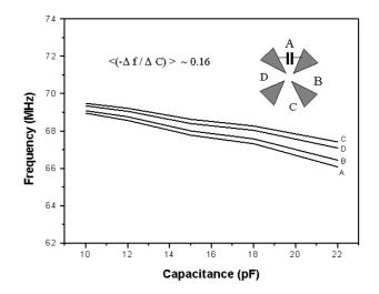
Figure 3: The variation of resonance frequency as a function of capacitance in the four quadrants of the RFQ  $\frac{1}{2}$  scale model. The value of  $R_p/Q$  is determined from  $\frac{\Delta f}{\Delta C}$ .
