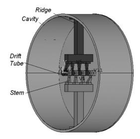
Figure 4: A schematic of IH-Linac tank.
