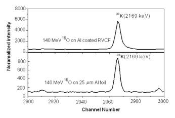
Figure 2: The normalized intensity of 2169 keV gamma ray from the decay of  ${}^{38}$ K produced from "thick" and "thin" aluminum targets.
