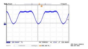
Figure 3: Filling pattern at the beginning of top-up injection. Filling pattern is identical to the shown pattern at the end of the test.
