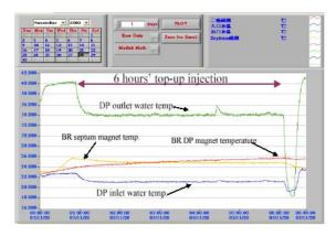
Figure 6: The temperature readings of dipole magnet and septum core under intermittence operation mode of injector at TLS.
