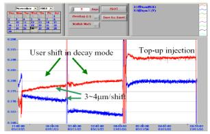
Figure 5: Reading of BPMs in the storage ring indicates the current-dependent effects. The reading of beam position can drift as much as 3-4  $\mu$ m in one user's shift, if the effect was calibrated correctly.
