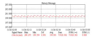
Figure 2: Zooming the top-up injection. The injection interval is 2 minutes, maximum beam current is 200 mA and the current bin is ~0.6 A.
