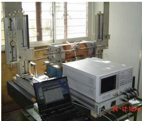
Figure 3: Bead-pull measurement setup for the field distribution analysis of the short technological model.
