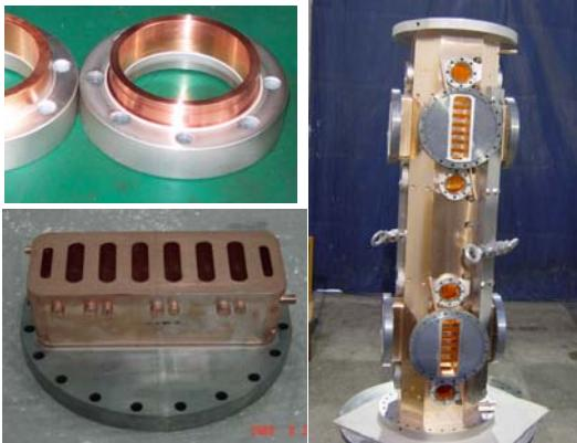
Figure 6: The 1.2m long full size model for brazing test with tuner and vacuum flanges.
