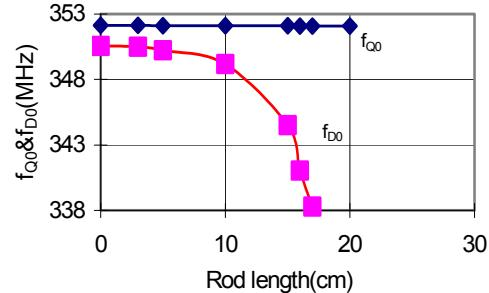
Figure 8: The measured dipole-rod effect on operating quadrupole mode and dipole mode.
