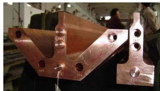
Figure 5: The water cooling channels of 1.2m long were drilled through the pieces and plugs were used to cover them on each end by brazing.
