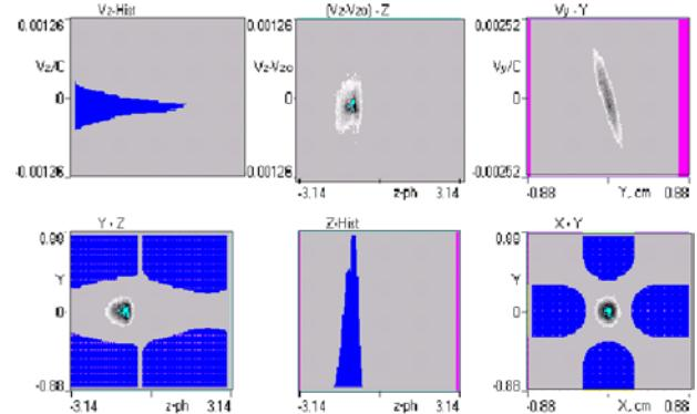
Figure1: LIDOS.RFQ simulation of beam bunch just ahead of the coupling gap.
