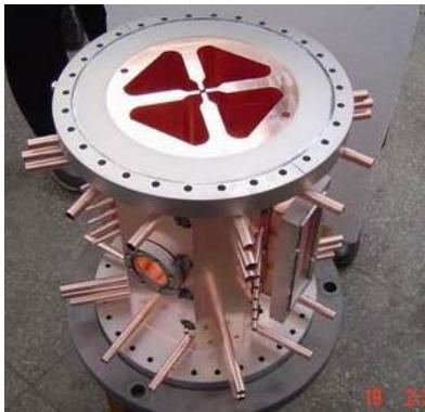
Figure 2: A Short RFQ technological model after final braze.
