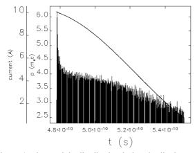
Figure 4: The particle distribution in longitudinal space at gun exit
