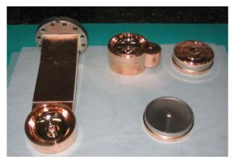
Figure 2: Some parts of the RF gun. (The coupler and the side cavity has been brazed to the first cavity and the second cavity respectively)
