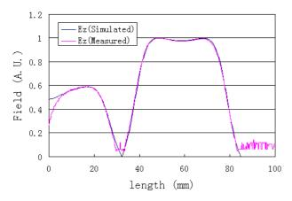
Figure 3: The field profile of RF gun at  $\pi/2$  mode.
