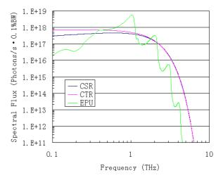
Figure 8: The THz radiation brightness from CTR, SR and EPU.
