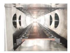
Figure 4: The magnet cover the Ni-plated Cu foil.
