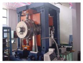
Figure 8: In-vacuum wiggler (4W2).
