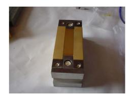
Figure 1: Diagram of half period of magnetic array of 4W2.
