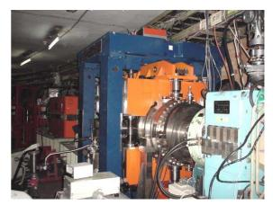
Figure 9: The in-vacuum wiggler to installed into BEPC storage ring.
