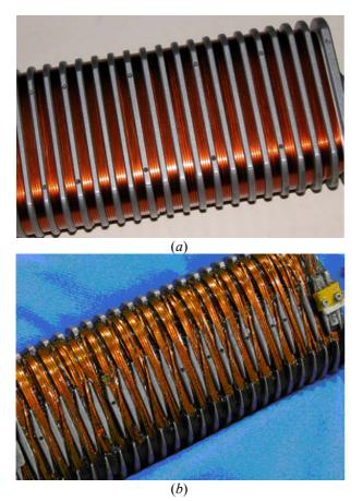
Figure 4: One core for the 12-period upper-half SCU was machined from low-carbon steel. (*a*): Bottom flat side of the core shows coilpacks and magnetic poles. (*b*): Top side shows additional cross-over windings, connecting every other coilpack by the conductor transition to the next period after complete winding of the 20 turns in one groove.
