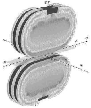
Figure 1: One 15-mm-period, 3-D model of the SCU used for the magnetic field calculations. Two steel cores (gray) are positioned to form a pole-gap height of 8 mm to accept the beam chamber. The core has grooves for 20-turn SC coils (*black*).
