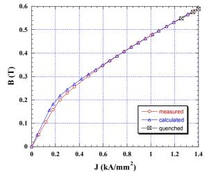
Figure 5: The vertical field for the upper-half SCU was measured at an approximate distance 3.6 mm from a magnetic pole. The calculated data, using the permeability data for the1008 low-carbon steel, gives slightly higher field values at low current densities.
