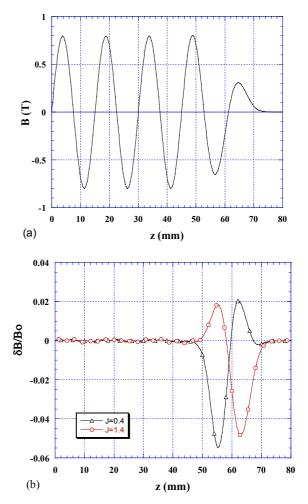
Figure 3: (a): The vertical fields, including the end, were calculated at a current density of 1.0 kA/mm<sup>2</sup> along the beam direction z of the SCU. The three end coils have 17, 10 and 3 turns instead of the nominal 20 turns. (b): At J = 0.4 and 1.4 the normalized field deviations from J = 1.0 are plotted.
