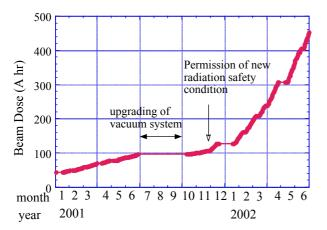
Figure 2: Accumulation of beam dose with time. The increase of beam injection in November 2001 brought a sudden change of stored beam current and rapid beam self-cleaning.
