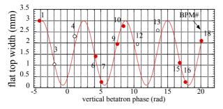
Figure 4: Flattop width of the aperture survey vs. the vertical betatron phase. The line is a 4th harmonic sinusoidal wave. The shaded circles and clear circles are critical locations face to SSS and LSS, respectively.
