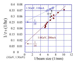
Figure 5: Vertical beam size ( $\sigma$ ) versus the beam lifetime at 1.0 GeV (circle) and 1.5 GeV (square). The points at [1/beam size] = 0 are considered to be  $1/\tau_R$ .
