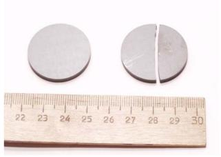
Figure 4: Picture of the boron carbide "Pure Tech" samples. Right – cracked sample after the test.
