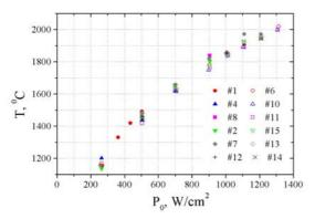
Figure 6: Maximum temperature of MPG6 graphite samples vs. the peak heating power density.
