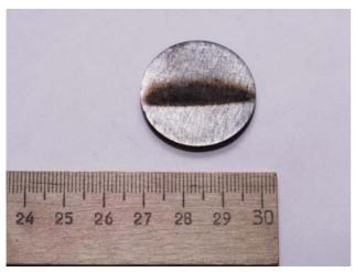
Figure 5: Picture of the glassy carbon sample after experiment.
