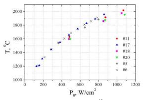
Figure 7: Maximum temperature of <sup>13</sup>C graphite vs the peak heating power density.
