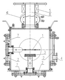
Figure 1: Experimental device. 1 – sample support. 2 – flanges, 3 – beam dump, 4 – pumping flange. 5 – magnetic correctors. 6 – optical windows, 7 – current outlets, 8 – beam channel.
