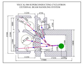
Figure 1: Beamlines layout for the superconducting cyclotron at Kolkata
