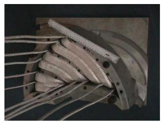
Figure 11: Trim coils wound on pole-tip.
