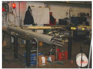
Figure 9: Vacuum jacketed and liquid nitrogen shielded cryogenic transfer lines under fabrication.
