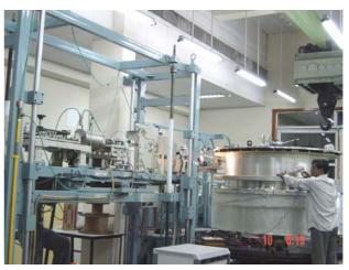
Figure 4: Superconducting coil winding in progress
