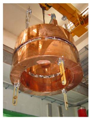
Figure 6: Cryostat bobbin with multilayer insulation and LN- 2 cooled radiation shield. Support links are also shown.
