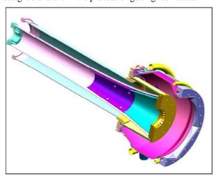
Figure 10: Computer generated model of inner and outer conductor of RF resonator with cooling lines.
