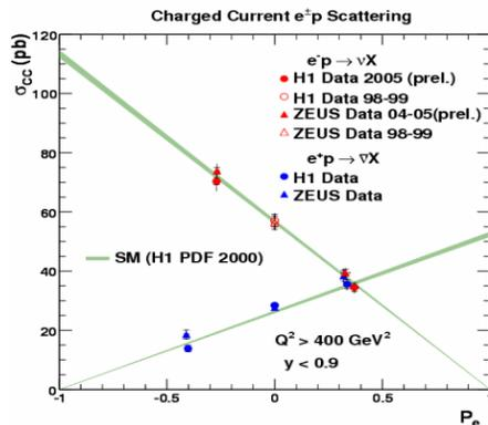
Figure 7: Measurements of the charged current cross section in HERA versus lepton beam polarization [28]
