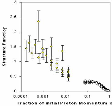
Figure 3: First measurement of ep scattering cross section versus  $x$  at HERA [24] including results of ref [4].
