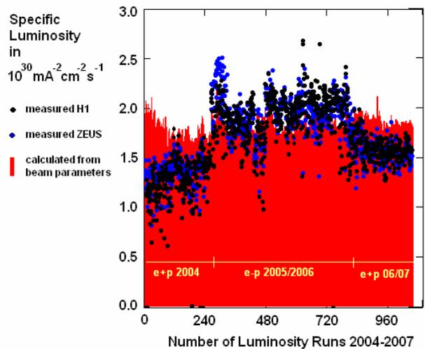
Figure 1: Specific Luminosity for HERA lepton proton collisions since 2004. The specific luminosity is significantly larger with electrons. Specific luminosity with positrons is recovered partly with tunes below the integer resonance in 2006/7.
