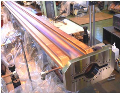
Fig. 1 Copper beam duct with two ante-chambers for tests.
