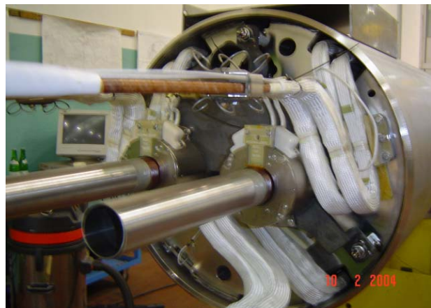
Figure 1: MCS fitted at one end of LHC Dipole.
