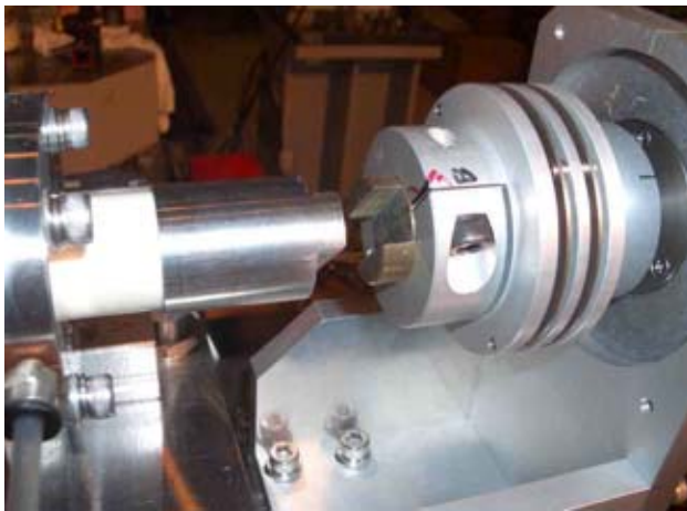
Fig.3. Coupling between the coil rod (left) and the encoder (right).
