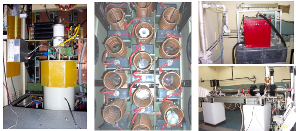
Figure 3: Left - Klystron modulator showing discharge thyatron with associated supplies, command charge thyatron above the main thyatron. Middle- Tuneable Pulse Forming network Right up- klystron assembly on high voltage deck. Right lower-waveguide system connected to LINAC input.
