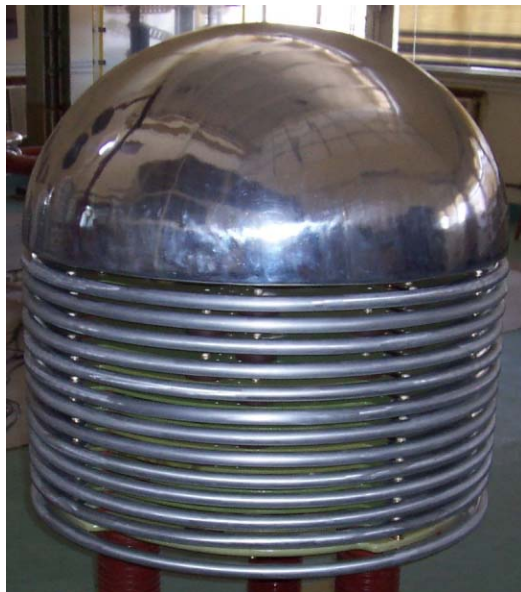
Figure 3: 300 kV multiplier stack assembly
