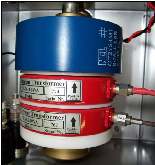
Figure 3: Re-trigger CTs in the droop compensation switch.
