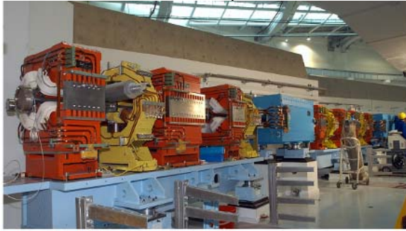
Figure 6: The sector machine in the tunnel.
