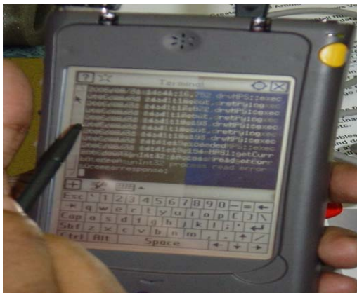
Figure 3: IOC running on arm based embedded system
