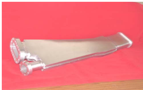
Figure 6: Prototype dipole vacuum chamber for TL-2.
