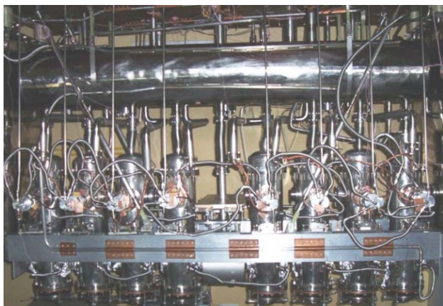
Figure 5. Eight resonators and a solenoid in first linac module ready to be loaded for a cold test.
