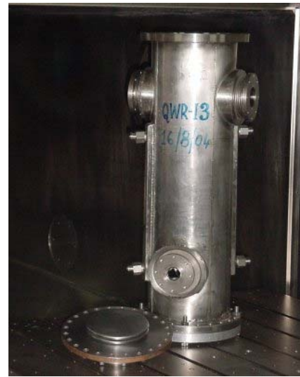
Figure 1: Indigenously built niobium quarter wave resonator with slow tuner bellows at IUAC.
