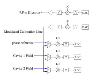
Figure 4: Insertion of phase calibration signal.
