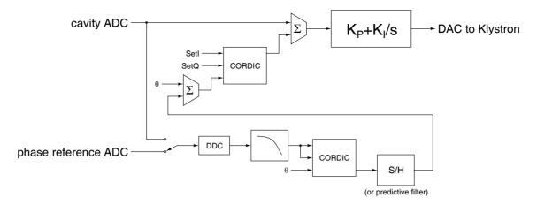
Figure 5: Digital signal processing of cavity and reference signals.
