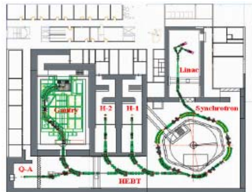
Figure 11: Layout of HIT (Heidberger Ionenstrahlen-Therapie) at Heidelberg.
