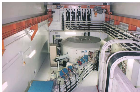
Figure 7: Normal conducting proton cyclotron by IBA at Kashiwa.
