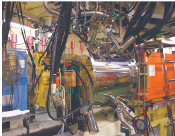
Figure 3: A superconducting wiggler installed between two bending magnets.
