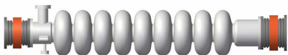
Figure 4: A nine-cell cavity for the main linac. HOM absorbers are on both sides.
