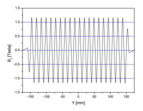
Figure 1: The calculated field profile.
