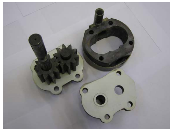
Figure 5 : The parts of liquid lead cogwheel pump.
