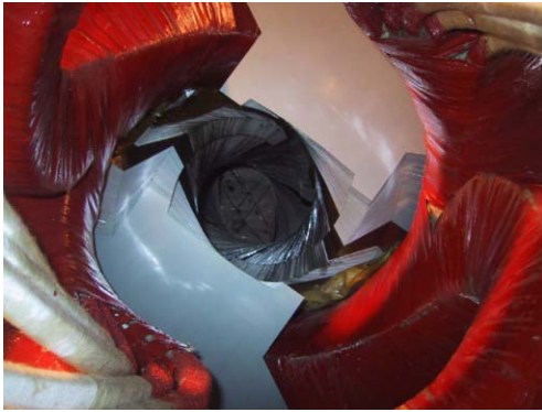
Figure 6: View down the magnet gap of the warm, iron-based helical partial Siberian snake of the AGS.
