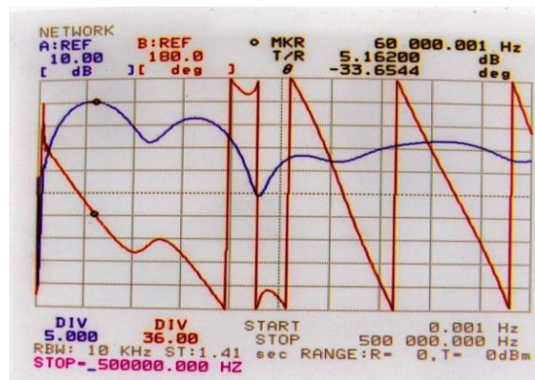
Figure 3: 10-tap FIR filter frequency response used in PF-AR multi-bunch feedback. (Blue line – amplitude response; red line – phase response).
