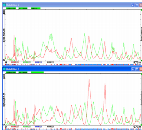
Figure 4. Top and bottom plots show the change in the beta-functions (red trace – horizontal, green - vertical) in pbar direction when EQ2 quad strength is changed by 1%.
