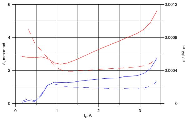
Figure 5: Compensated emittance (solid) and quality factor (dashed) vs. peak current of Gaussian bunch. Upper (red) curves take slice emittances into account.
