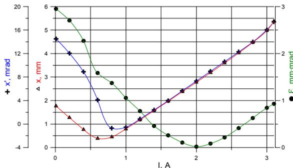
Figure 2: Beam parameters vs. beam current: rms-size, its derivative and emittance.
