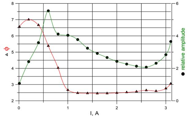
Figure 3: Charge phase and relative amplitude vs. beam current.
