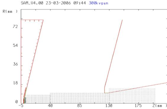
Figure 1: The geometry of the basic gun, red solid lines are electrodes.
