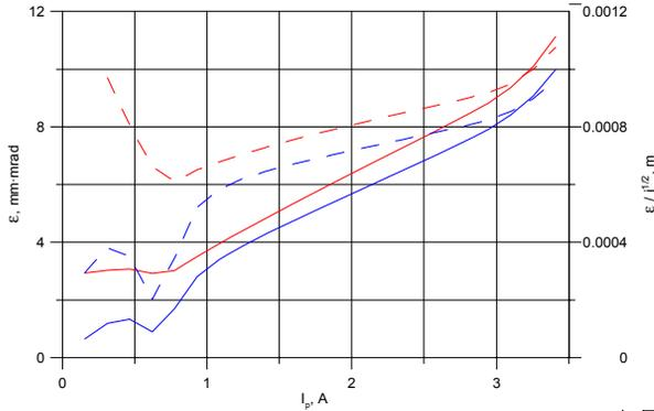
Figure 4: Non-compensated emittance (solid) and  $\varepsilon/\sqrt{j}$  (dashed) vs. peak current of Gaussian bunch. Upper (red) curves take slice emittances into account.
