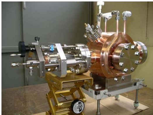
Figure 1: The third harmonic cavity.
