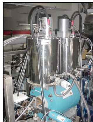
Figure 1. View of the High Temperature Superconducting ECR Ion Source, PKDELIS
