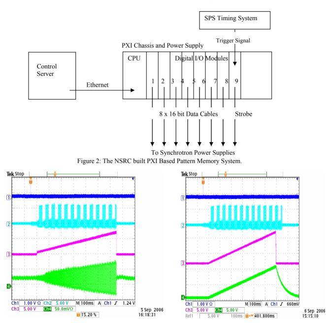
Figure 3: Input and output signals of the synchrotron RF amplifier system. Channel 1, the 1 cycle trigger signal. Channel 2, PM data output example. Channel 3 RF voltage envelope generated by the data. Channel 4, the RF signal at 118MHz.
