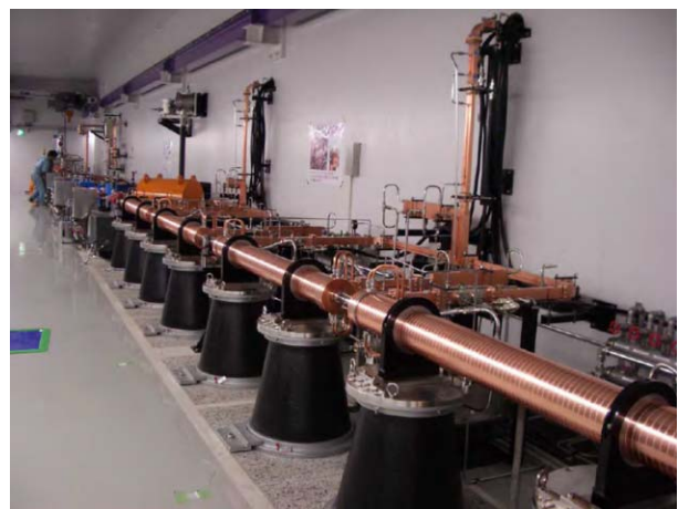
Figure 2: A photograph of the C-band accelerator. This view is from the downstream of the C-band accelerator.
