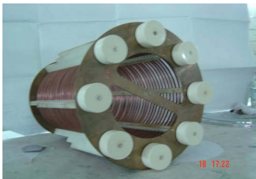
Figure 9: Assembly of RF Choke & HV Filter capacitors.
