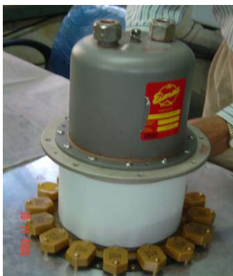
Figure 10: Assembly of Screen by-pass capacitors.
