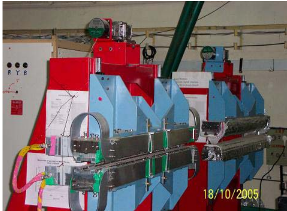
Fig. 5 Photograph of two Undulator segments with the field mapping system and corrector coil mounted
