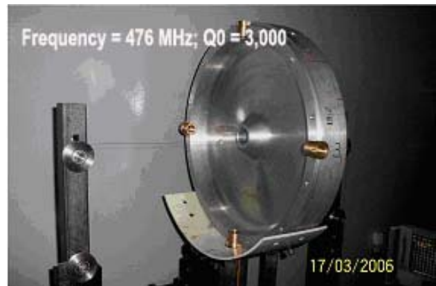
Fig 2 Aluminium prototype of pre-buncher cavity
