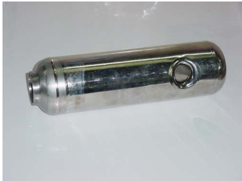
Figure 5: A repaired Drift Tube assembly.
