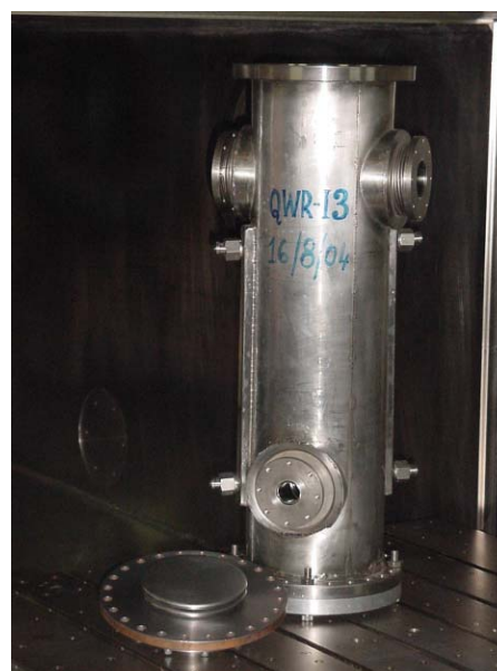
Figure 2: One, of the two, fully indigenously built QWRs at IUAC along with its niobium slow tuner bellows.
