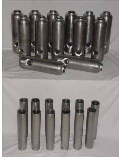
Figure 4: Loading Arm (below) and Drift Tube (top) assemblies.
