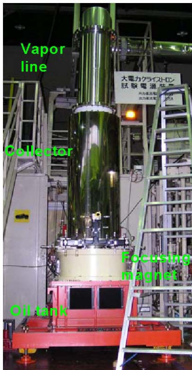
Figure 5: Test facility for E3762
