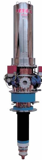
Figure 7: 170-GHz, 1-MW gyrotron E3993
