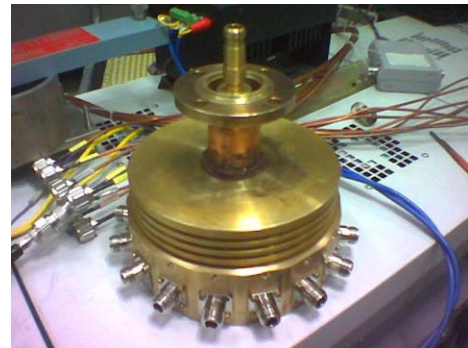
Figure 3: 16 way power combiner/divider structure
