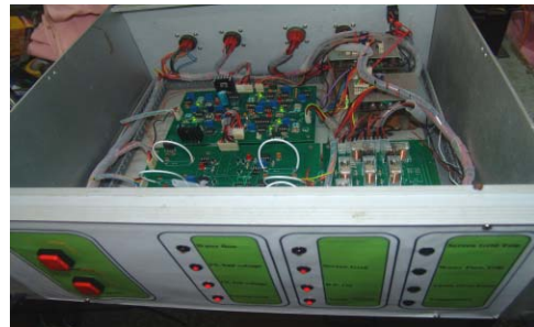
Figure 5: Interlock and Protection circuit.
