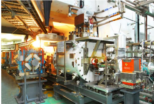
Figure 5: A superconducting cavity in installation.
