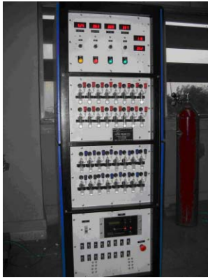
Figure 3: Front view of the 4-component gas mixing unit with 16 output channels.
