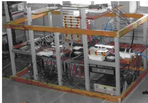
Figure 2: Muon tracking setup using RPC stack.
