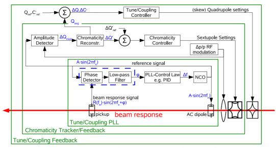
Figure 3: Nested loop scheme required for a coherent control of tune, coupling and chromaticity.
