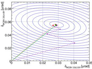
Figure 1: SVD residual contour: The perfect correction (solid green), the correction with optics error (dotted red) and COD calibration errors (dashed violet) are indicated. The contour lines correspond to constant values of the residual orbit error r. The correction is based on a regular FODO lattice (LHC arc) and shows the projection of two selected COD settings.
