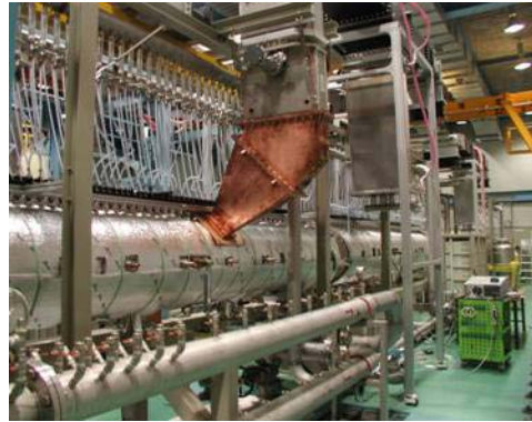
Figure 4: The PEFP 20 MeV DTL.
