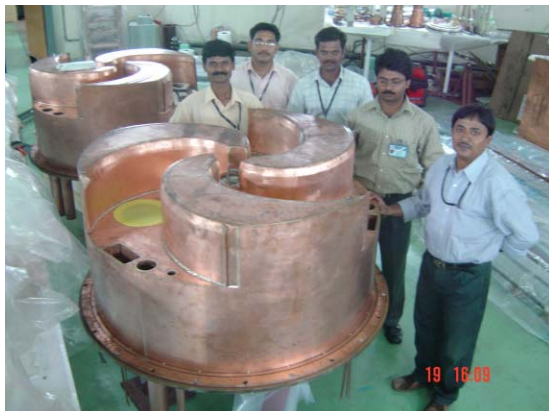
Figure 20: RF liner assemblies ready for installation.
