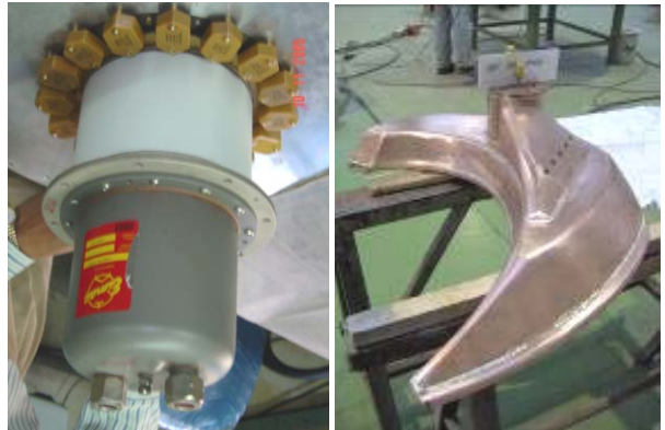
Figure 17: Assembly of screen bypass capacitor with tetrode tube (left) and upper half of one of the three dees (right).
