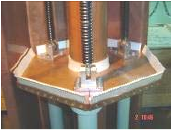
Figure 18: Sliding short assembly with Be-Cu contact fingers.
