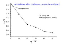
Figure 4: Acceptance after cooling vs. proton bunch length.
