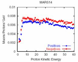
Figure 3: Efficiency of muon collection at the exit of the Study 2a front end versus proton driver energy.
