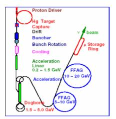
Figure 2: Schematic layout of a neutrino factory.
