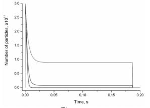
Figure 6: Expected  $U^{28+}$ -beam intensity evolution in SIS18 during a 4 Hz booster sequence, calculated with StrahlSim. It was assumed that only 8 % of the gases desorbed inside the "desorption" scrapers are able to interact with the revolving beam. The different curves indicate different steps of the UHV system upgrade.
