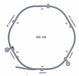
Figure 2: Distribution of the injection-, extraction- and transfer systems and the RF systems for acceleration and bunch compression in the six straight sections of SIS100
