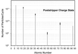
Figure 5: Present status of maximum number of particles of ions with different atomic numbers and intermediate charge states accelerated in SIS18.
