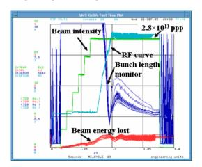
Figure 5: 'NuMI only' cycle in Main Injector
