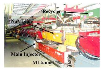
Figure 2: A photo of the Main Injector tunnel in the MI-60 region, showing the NuMI extraction line between the Main Injector at the bottom and the Recycler on top.
